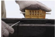
2. Use the flat-head screwdriver to punch out the hinge from the inside of the container.
