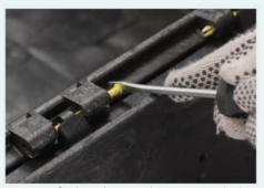
2. Use a flathead screwdriver to push the new pin into the hinge location.
