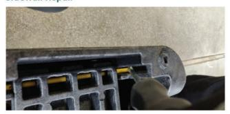
1. Use a flat head screwdriver to push the rod towards the open hole at one side of the container.
