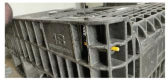
3. Push the rod through the hole to remove it. Once the rod is fully removed from the container, you can lift off the side wall and replace it if necessary.
