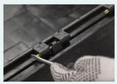
1. Insert the flathead screwdriver on the back side of the hinge and move the hinge pin out of its location.
