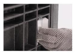
3. Put the new latch in place. Push down on the latch and it will snap into place. Latch replacement is the same for the sidewall and the access door.
