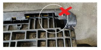
4. Push a new rod through the hole and move it with your fingers to put it into position. To ensure proper functionality, push the rod through completely until it reaches the other end of the bin.
