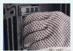
2. Push the latch over so it disengages from the tab and the latch will be able to be removed. Remove the latch.
