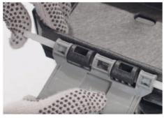
3. Remove the hinge and slide the new hinge into the hinge location. Use a screwdriver or fingers to push the two hinge pins towards the center of the hinge.
