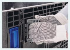
3. Put the new latch in place. Push down on the latch and it will snap into place. Latch replacement is the same for the sidewall and the access door.
