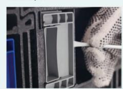
1. Insert the flat-head screwdriver in between the latch and the tab that is holding the latch in place.
