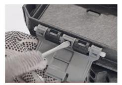
2. Use a flat-head screwdriver to separate hinge pins in the center section of the hinge. Use the pliers to pull the hinge pin away from the center section. Stop when the end of the hinge pin is in line with the outer section of the hinge.
