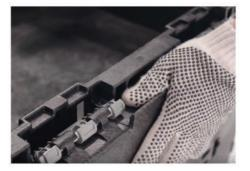
4. Press down and the new hinge will snap into place. Open and close door to insure correct fit.
