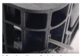
2. Once the rod is out a few inches, the operator should be able to pull the rod out the rest of the way.
