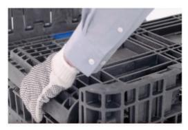
3. Remove hinge rod and sidewall to replace with new ones.
