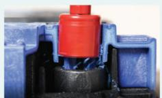
2. Drill out all snapp collars. Make sure to only drill out the stringer/runner portion. Once all connections are released, you can easily remove the runner/stringer.
