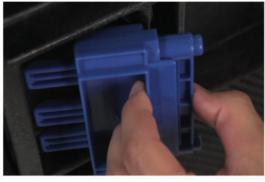
3. Put a new latch in to place by pushing it together and bringing it in the right position.
