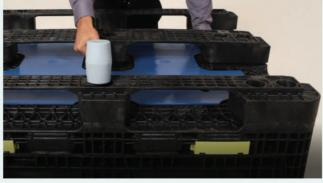
4. Put the new stringer/runner into place. Strike each foot with a rubber mallet to engage the stringer/runner.
