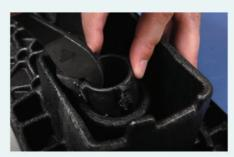
3. With a side cutter, remove all snap tabs by cutting them into smaller pieces.
