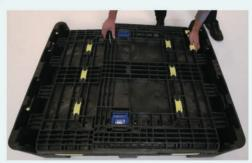
2. Remove all panel clips to fully release the side wall.
