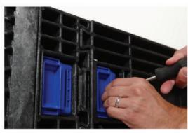
1. Use a flat-head screwdriver to push the latch together.
