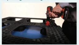
1. Insert the drill with a 50mm hole saw into the holes at the connection points.
