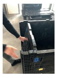
Erect the two short side walls one after the other by grabbing the opening und pushing the wall into position. The blue latches of the short side walls will snap into the openings at the inner side of the long side walls. The side walls need to be erected evenly to a centered position to ensure that they snap-in smoothly.
