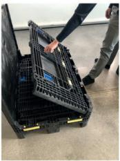
In order to erect the container, grab the side wall with two fingers and pull it into position. There is an opening at the side walls specifically intended for this purpose. Repeat the process on the opposite side.
