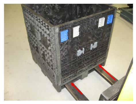
Do not slide containers off of fork tines. Fork truck should come to a complete stop prior to off loading the container.
