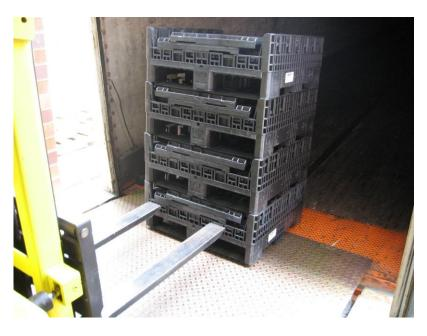
Pushing the containers into trailers with fork truck may cause damage or injury.
