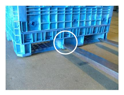
If fork tines are not properly aligned, they will damage the base.
