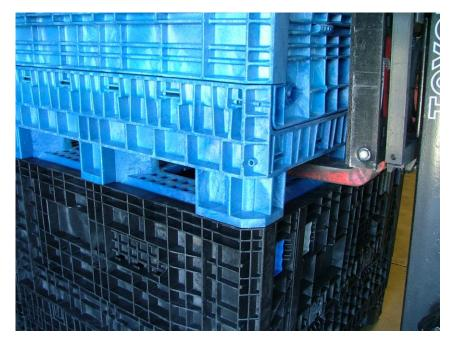
Bulk bins should be stacked securely on each other to support worker safety and eliminate bin damage. To properly stack, place bin directly on top on lower bin, with no sliding.
