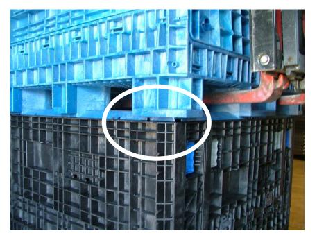
If bins are not nested properly, they will cause damage to bins and might cause stack failure and worker safety issues. Make sure you are matching up the correct sides. (48" vs 45")
