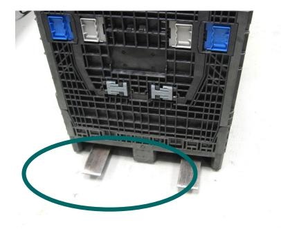
Fork tines should be fully under the bin supporting the weight load. Fork tines should not protrude beyond the bin footprint. This can cause damage to other containers during stacking.
