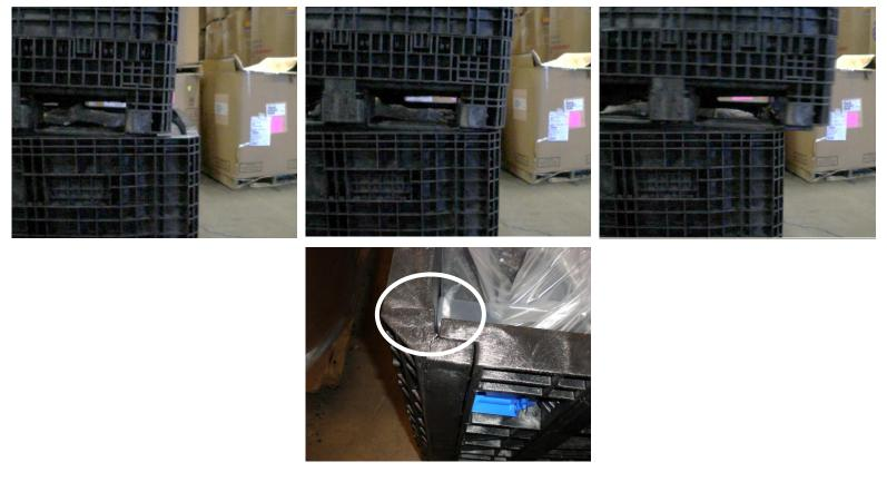
While stacking bins, do not use the back wall of the lower bin to stop or locate the bin on top. Sliding the top bin into the back wall of the bin below or running across it, will cause damage to the upper corner sidewall.
