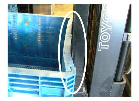
Mast of fork truck must be properly aligned with bulk bin during handling.
