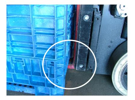
Fork tines should be under bin to fully support unit load.
