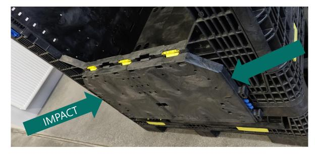
Avoid impact of open access doors from the side. Impacting the access door from the front with a forklift may cause damage.
