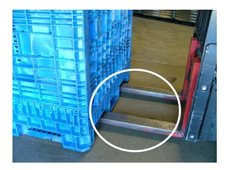
If fork tines are not fully under the bin (short forking), it will increase risk of bin falling and damage to bin.
