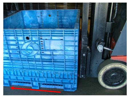
Pushing bins across the floor will damage bins and facility.
